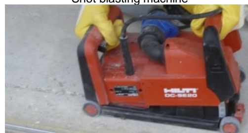
A double disc rotary saw for grooving
