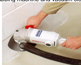
Grinding of edges with diamond discs
