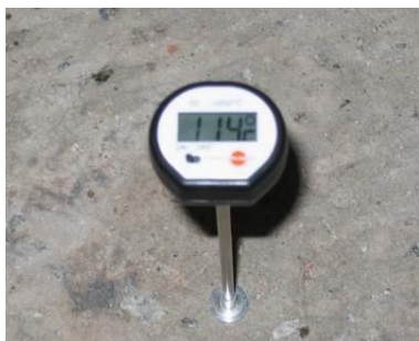
Surface temperature > 10°C
