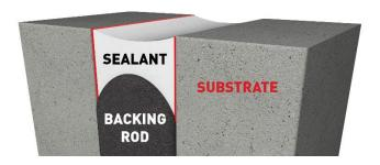
The optimal bond thickness for this product is at least 2 mm for the elastic properties to come to full justice.
