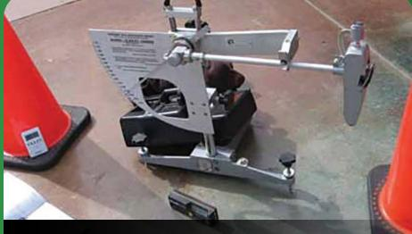
Pendulum test in progress
