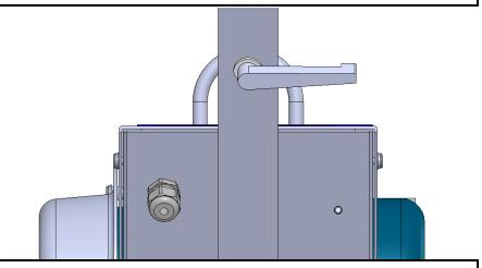
8. Tighten the hand screw securely when in required position.
