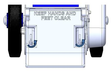
1. Turn the handles to loosen the bottom
