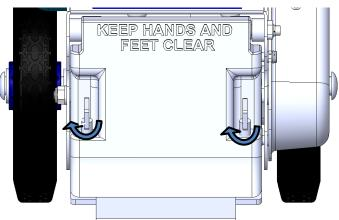
4. Tighten the handles evenly while ensuring the blade is straight.
