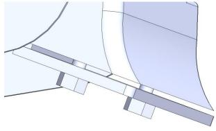
2. Slide the blade through the gap and in between the two bolts until it hits the back stop.
