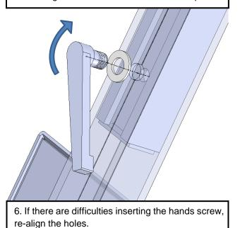
7. To adjust, loosen the hand screw enough until the handle can move up and down.
